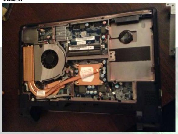
The W110ER, has 1 cooler, with 2 cooling pads, 1 for gpu the other for the cpu, and 1 fan, common, located at the end of the coolers extremity. The first thing to notice is that the laptop is incredibly silent while working. In stress, even though it is a noisier it's nothing to be alarmed about, or to take too seriously.
